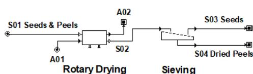
**Figure 8: Drying of tomato pulp and separation of seeds and peels**
