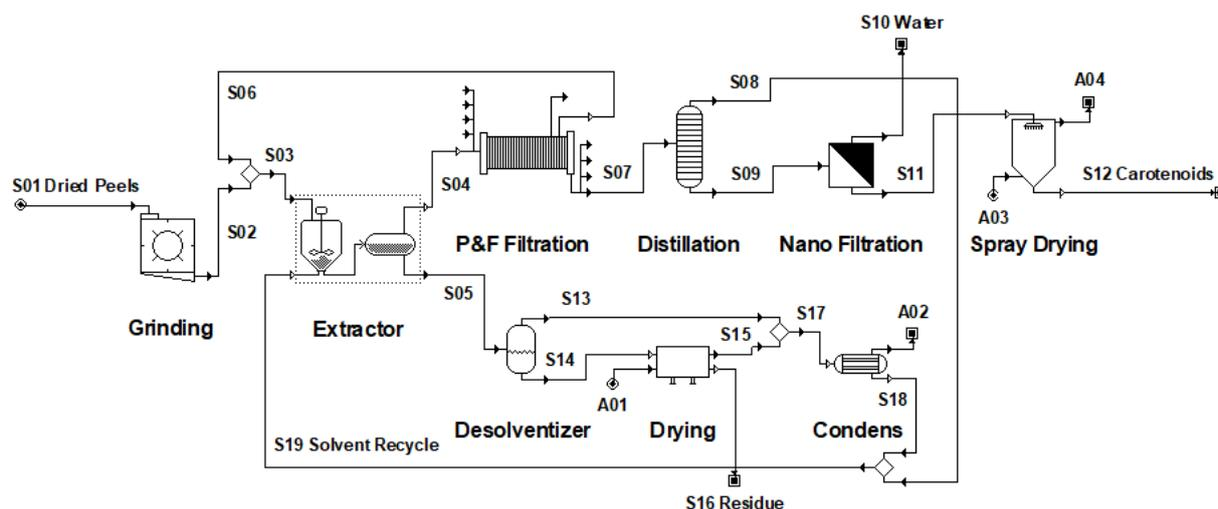
**Figure 10: Carotenoid extraction process from dried tomato peels**
