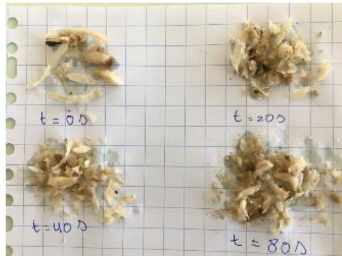
Figure 5: Processed chicory fibre of particle size distribution of various grinding times (20s, 40s, 80s), depicted on 1 cm 2 graphing paper.
